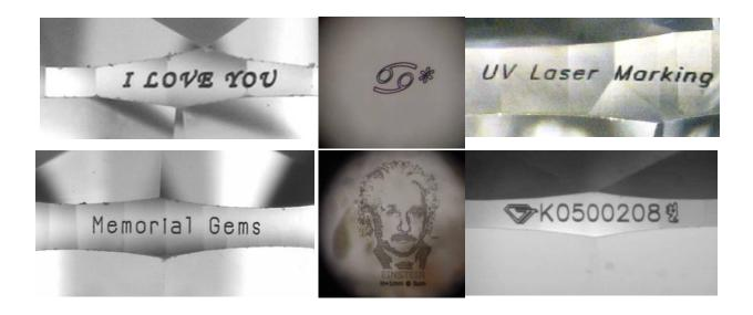
By modifying the iris or the power, one can modulate the marking to be lighter or darker.
